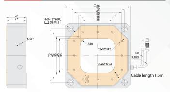
Note: Max driving voltage could be -20V $\sim$ 150V, recommended voltage 0 $\sim$ 120V for long-term, high-reliability operation. Technical data is measured by CoreMorrow E00/E01 series piezo controller.
