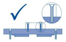
FIG.7 The correct bolt connection
