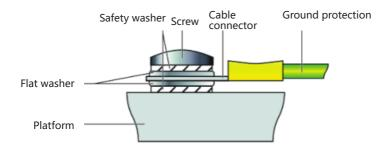
FIG. 3 Grounding protection diagram
