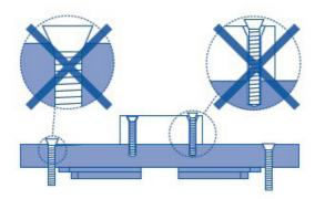
FIG.8 Inappropriate bolt selection
