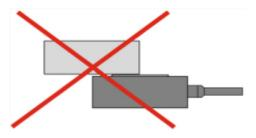
FIG.6 Do not mount long loads on one side of the platform
