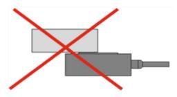
Do not load longer loads and add to the side of the piezo stage
