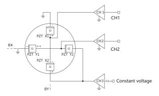
Piezo tilt stage(two-axis motion) is based on parallel kinematic design with coplanar axis and moving platform. Four piezo actuators are placed at a 90° angle interval, paired differential control distribution. Two pairs of differentially driven actuators provide the highest achievable angular stability over a wide temperature range. Its tilt motion is achieved by two pairs of piezo actuators in a push-pull motion, controlled by a bridge connection circuit.
