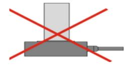
It is forbidden to mount the load on one side of the moving platform, which will cause serious damage to the product, as shown in the figure below.
