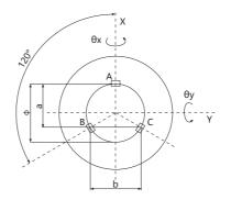
S23 has build-in three piezo actuators connected in parallel to provide the top ring motion. For vertical positioning (piston movement), it requires a controller with only one drive channel and three drive channels when it is in Z-direction and tip/tilt motion. The deflection angle of S23 Tip/Tilt Platform can be calculated as follows:
