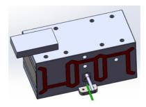
FIG.3 The load is applied to the center of the moving surface
