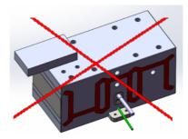
FIG.5 Do not mount long loads on one side of the platform
