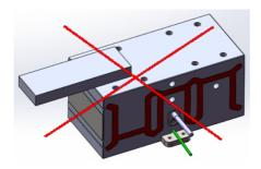
FIG.4 Try not to let the position of the center of gravity far exceed the active platform
