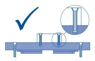
FIG.6 The correct bolt connection
