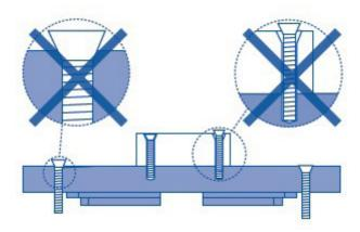
FIG.7 Inappropriate bolt selection
