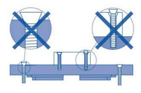
FIG.8 Inappropriate bolt selection
