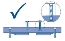
FIG.7 The correct bolt connection
