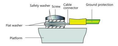
FIG. 3 Grounding protection diagram
