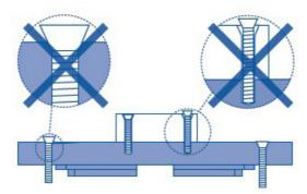
Figure 8 Incorrect connection
