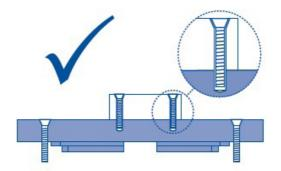
Figure7 Correct connection
