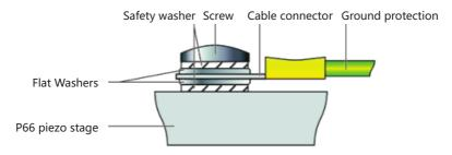
Figure 2 Ground protection diagram
